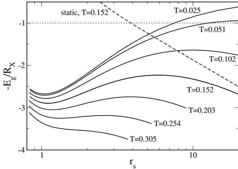
$R_X > \min[\mu_{eh}(r_s, T)] = \min[-E_g(r_s, T)] \Rightarrow X \text{ phases unstable against EHL}$
