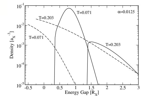
above  $T_c(E_g) \exists (E_g, T)$ -range where Xs prevail over unbound electrons and holes (halo) & give rise to additional scattering channel (e-X, h-X)  $\Rightarrow$  resistivity anomaly
