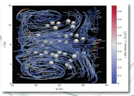
Plasma flow around and charge distribution of a dust cluster in a rf discharge DOI: 10.1063/1.5021316
