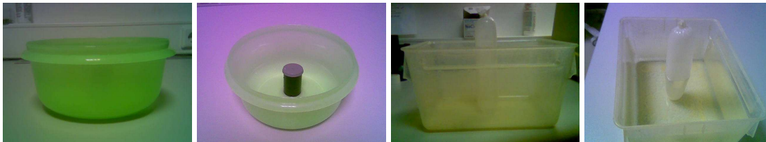
Figure 4.1: Left: water filled phantom consisting of a round plastic box (diameter 18.9cm), inside an air filled film can (inner diameter 3cm) is glued to the bottom of the box; Right: water filled phantom consisting of a rectangular plastic box (bottom: (22×16)cm, top: (25.4×19.5)cm) where an air filled condom is glued to the bottom, but can move freely inside the water.
